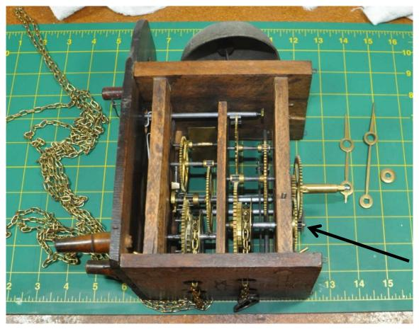
The motion works are driven from the first wheel not the minute arbor.
