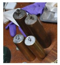
Noticed some days time chain ran out quicker than others. It was slipping over worn pins. Replaced pins. Should do same on strike side.
