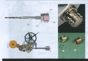
The winding crown is made of 24 gold rivets (133) inserted inside a drilled tube (170) and tightened by a tiny cabochon (159).
