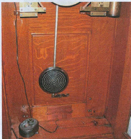
Early Howard watch clock with hand-wound cable and weight-driven movement.
