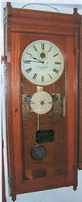
Early Howard watch clock with hand-wound cable and weight-driven movement.
