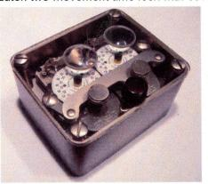
Eaton time lock with front cover installed. Note the magnifier lenses positioned above each movement dial.
