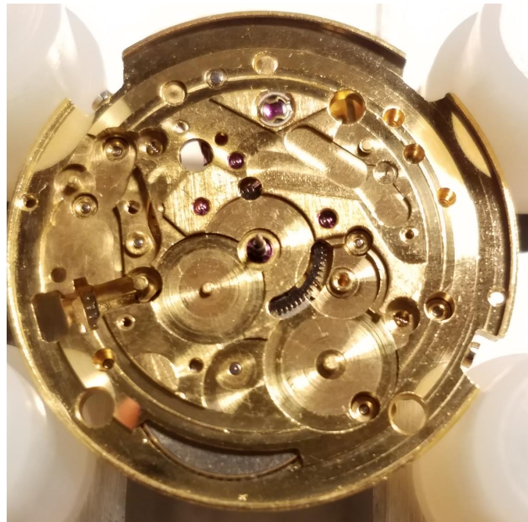
Dial side clean and ready for reassembly
