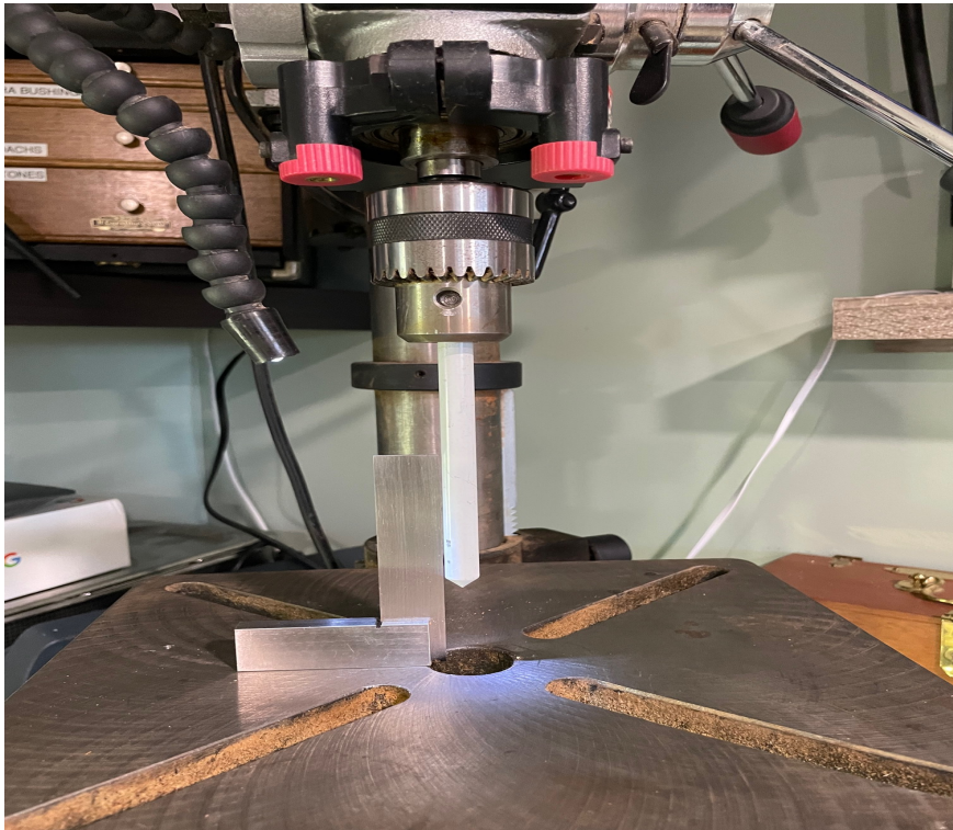
Checking with Square
