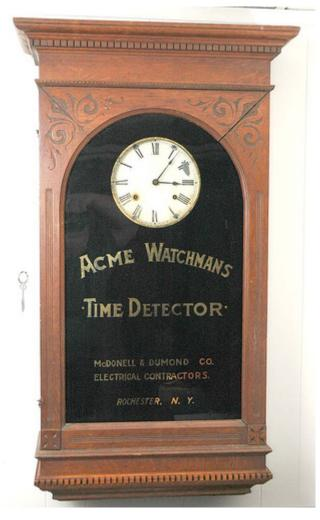
Owned by a fellow NAWCC collector in KY. D. Phelps. I stole his pic from the NAWCC site. The lettering on the glass suggests to me that it was reconditioned and resold by "Acme". it is a 20 station and the inside ST movement is identical to all the Holtzers I have seen. The 80 beat 15 day Seth Thomas independent of watchmans device dial powered by ST #10.
