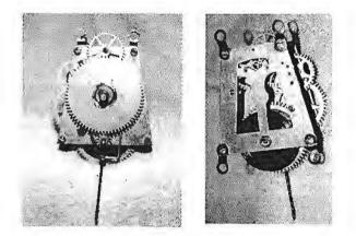
This movement was part of a box of movements that I acquired. It is a Pendulum movement and VERY heavy for it's size. Large gear on front of movement with arbors about 1 3/8" center to center. Time only. Seth Thomas and 3 1/2 are the only markings. Can you help identify what it may go to? Thanks, Bill Maune
