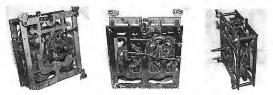
This movement was part of a box of movements that I acquired. It is a weight driven movement and VERY heavy. The front and back plates are very thick and are attached with pins instead of screws and nuts. Single hammer chime. Verge and some parts are missing. No names or markings can be found. Can you help identify what it may go to? Thanks, Bill Maune
