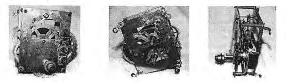
This movement was part of a box of movements that I acquired. It is a hair spring movement The front has a very large (Chuck) for the hands. Arbors are about 1 1/4" center to center with the winding arbor about the 2 o'clock position. Hair Spring and some parts are missing. It says made for The Bristol Co. Waterbury Conn by Seth Thomas. Also No. 402 BB 24H. Can you help identify what it may go to? Thanks, Bill Maune
